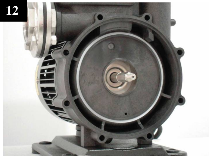
Remove the rubber from the stationary part.
