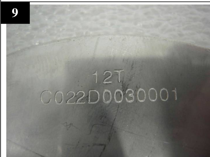
Identify the impellers – TQ3700, 2 impellers in same size, Parts# C022D0030001.
