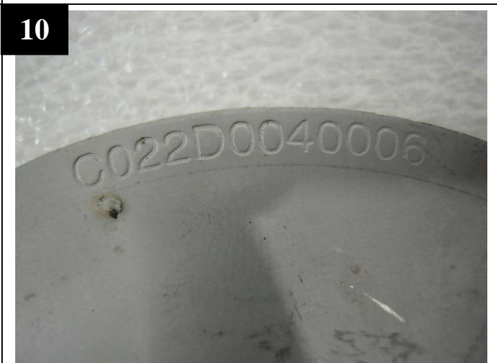
Identify the impellers – TQ2200, 1 st stage, Parts# C022D0040006. 2 nd state Parts# C022D0030001.
