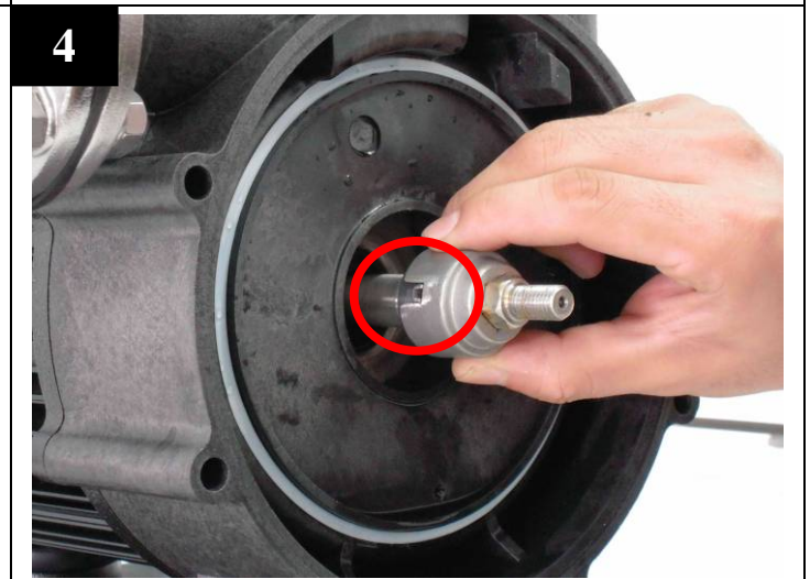
Before press in rotary parts, insert the sleeve through the hex shaft aligning the slots on sleeve to tabs on washer.
