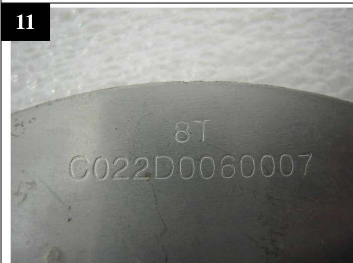
Identify the impellers – TQ1500, 1 st stage, Parts# C022D0040006. 2 nd state Parts# C022D0060007.
