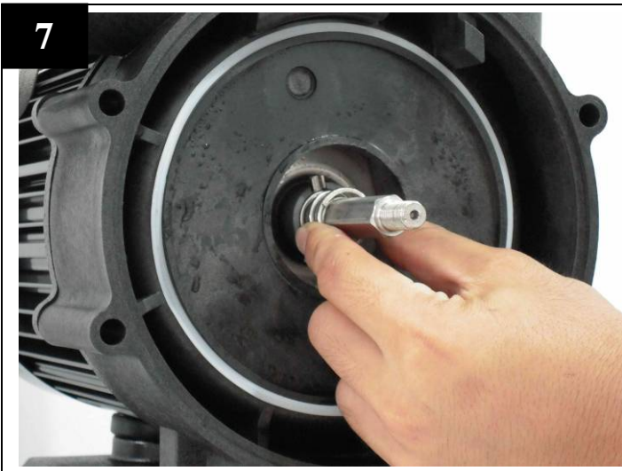
Place the spring onto rotary parts.
