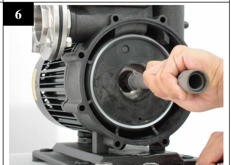
Before press in rotary parts, insert the sleeve through the hex shaft aligning the slots on sleeve to tabs on washer.
