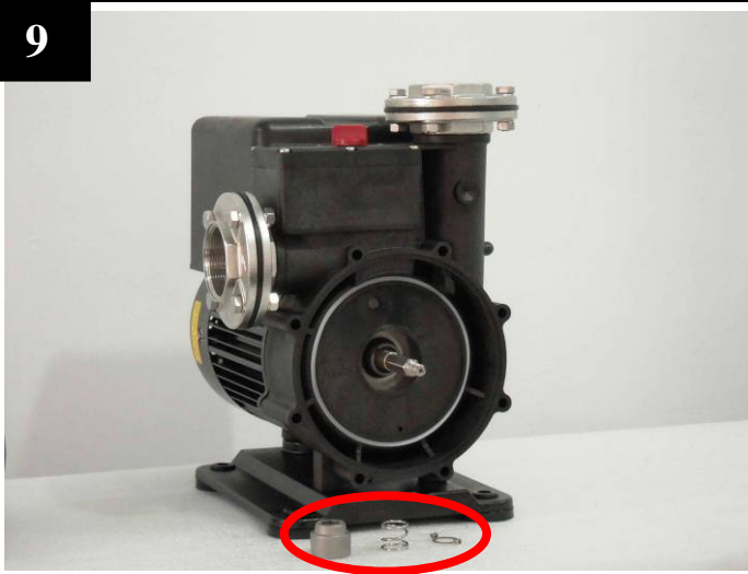
Remove the sleeve, spring and washer. (refer the red circled parts)
