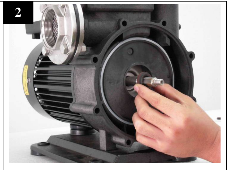
Place the stationary parts in position
