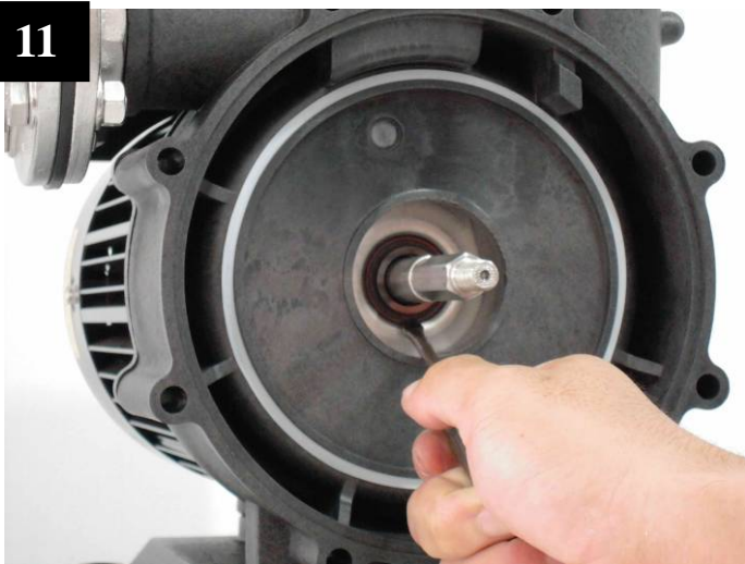
Remove the stationary part.
