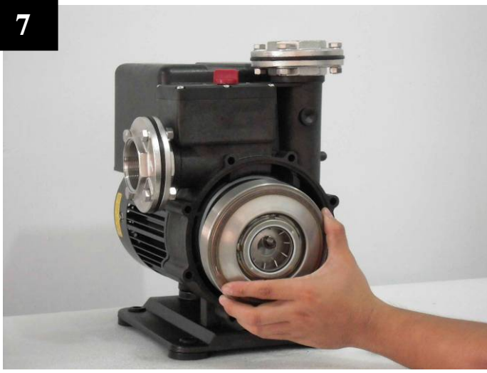
Remove the intermediate chamber kit.
