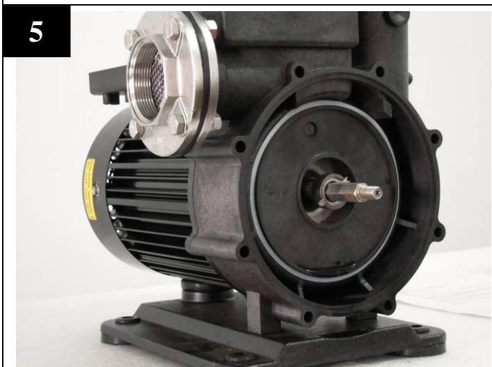
Remove the sleeve before press in rotary parts.
