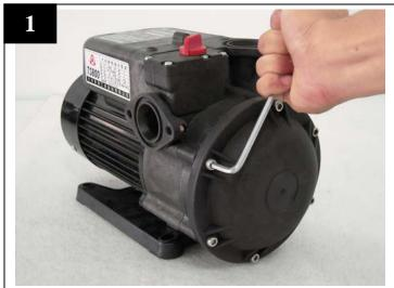
Using Allen wrench (metric size) to remove the 6 stud bolts.
