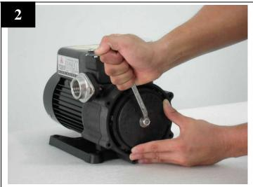
Using wrench to remove the stud bolt.
