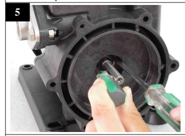
Remove the rotary parts of mechanical seal.
