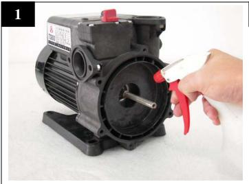
Spray water on the shaft as lubrication.
