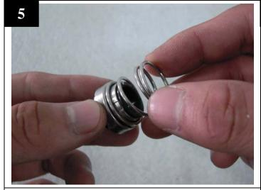
Place the spring onto rotary part.
