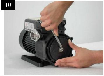
Place back all impellers, sleeves and intermediate chamber in order.
