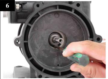
Remove the stationary part of mechanical seal.
